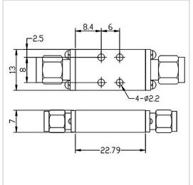
RF Solution offer a wide selection of Low Pass Filter for global customers. LPF-DCG23.6A-S is a Low Pass Filter in Frequency Range of DC~22.5 GHz. It is made of high quality materials under a high standard, the 3dB Cut-off of this product is 23.6 GHz, Insertion Loss Max is 1.3 dB and Rejection Min is 25dB@21.6GHz / 50dB@24.3-GHz. The component has a good working performance and stability, it is ideal for handling a Rated Power of 50 W.
