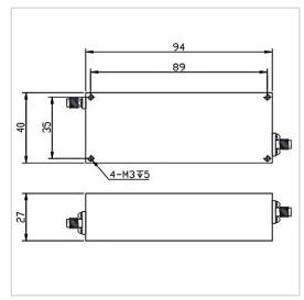
RF Solution offer a wide selection of Low Pass Filter for global customers. LPF-DCM1600A-S is a Low Pass Filter in Frequency Range of DC~1600 MHz. It is made of high quality materials under a high standard, the Insertion Loss Max of this product is 2.0 dB, Rejection Min is 40dB@1696-11000MHz and VSWR Max is 2.00. The component has a good working performance and stability, it is ideal for handling a Rated Power of 20 W.
