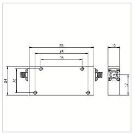
RF Solution offer a wide selection of Low Pass Filter for global customers. LPF-DCM2000A-S is a Low Pass Filter in Frequency Range of DC~2000 MHz. It is made of high quality materials under a high standard, the Insertion Loss Max of this product is 1.0 dB, Rejection Min is 50dB@2600-6000MHz and VSWR Max is 1.50. The component has a good working performance and stability, it is ideal for handling a Rated Power of 40 W.
