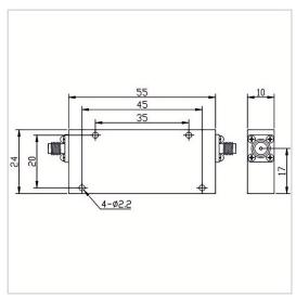
RF Solution offer a wide selection of Low Pass Filter for global customers. LPF-DCM2200A-S is a Low Pass Filter in Frequency Range of DC~2200 MHz. It is made of high quality materials under a high standard, the Insertion Loss Max of this product is 1.5 dB, Min 10dB@2400MHz Rejection is 60dB@2650-7000MHz and VSWR Max is 1.50. The component has a good working performance and stability, it is ideal for handling a Rated Power of 10 W.
