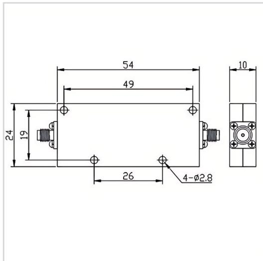
RF Solution offer a wide selection of Low Pass Filter for global customers. LPF-DCM2700A-S is a Low Pass Filter in Frequency Range of DC~2700 MHz. It is made of high quality materials under a high standard, the Insertion Loss Max of this product is 1.5 dB, Rejection Min is 50dB@4000-8000MHz and VSWR Max is 1.50. The component has a good working performance and stability, it is ideal for handling a Rated Power of 10 W.
