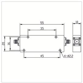
RF Solution offer a wide selection of Low Pass Filter for global customers. LPF-DCM2970A-S is a Low Pass Filter in Frequency Range of DC~2970 MHz. It is made of high quality materials under a high standard, the Insertion Loss Max of this product is 1.0 dB, Rejection Min is 50dB@3960-9900MHz and VSWR Max is 1.50. The component has a good working performance and stability, it is ideal for handling a Rated Power of 40 W.
