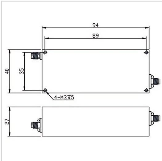
RF Solution offer a wide selection of Low Pass Filter for global customers. LPF-DCM4200A-S is a Low Pass Filter in Frequency Range of DC~4200 MHz. It is made of high quality materials under a high standard, the Insertion Loss Max of this product is 2.0 dB, Rejection Min is 40dB@4452-21000MHz and VSWR Max is 2.00. The component has a good working performance and stability, it is ideal for handling a Rated Power of 20 W.
