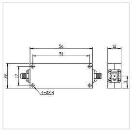
RF Solution offer a wide selection of Low Pass Filter for global customers. LPF-DCM4500A-S is a Low Pass Filter in Frequency Range of DC~4500 MHz. It is made of high quality materials under a high standard, the Insertion Loss Max of this product is 2.0 dB, Rejection Min is 40dB@4452-21000MHz and VSWR Max is 2.00. The component has a good working performance and stability, it is ideal for handling a Rated Power of 20 W.
