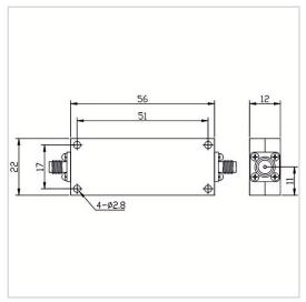
RF Solution offer a wide selection of Low Pass Filter for global customers. LPF-DCM5150A-S is a Low Pass Filter in Frequency Range of DC~5150 MHz. It is made of high quality materials under a high standard, the Insertion Loss Max of this product is 2.0 dB, Rejection Min is 50dB@6000-16000MHz and VSWR Max is 2.00. The component has a good working performance and stability, it is ideal for handling a Rated Power of 15 W.
