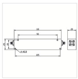
RF Solution offer a wide selection of Low Pass Filter for global customers. LPF-DCM5800A-S is a Low Pass Filter in Frequency Range of DC~5800 MHz. It is made of high quality materials under a high standard, the Insertion Loss Max of this product is 2.0 dB, Rejection Min is 40dB@6148-18000MHz and VSWR Max is 2.00. The component has a good working performance and stability, it is ideal for handling a Rated Power of 20 W.
