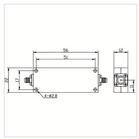
RF Solution offer a wide selection of Low Pass Filter for global customers. LPF-DCM6000A-S is a Low Pass Filter in Frequency Range of DC~6000 MHz. It is made of high quality materials under a high standard, the Insertion Loss Max of this product is 2.0 dB, Rejection Min is 70dB@9000-18000MHz and VSWR Max is 2.00. The component has a good working performance and stability, it is ideal for handling a Rated Power of 20 W.
