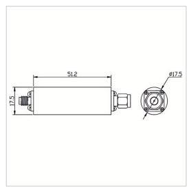
RF Solution offer a wide selection of Low Pass Filter for global customers. LPF-DCM8000A-S is a Low Pass Filter in Frequency Range of DC~8000 MHz. It is made of high quality materials under a high standard, the Insertion Loss Max of this product is 0.35 dB, Rejection Min is 25dB@9600MHz / 55dB@15000MHz and VSWR Max is 1.50. The component has a good working performance and stability, it is ideal for handling a Rated Power of 50 W.
