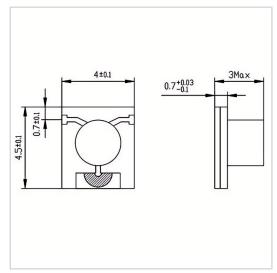
RF Solution offer a wide selection of Microstrip Isolator for global customers. MG0445-07 is a Microstrip Isolator in Frequency Range of 18.5~25.0 GHz. It is made of high quality materials under a high standard, the Insertion Loss Max of this product is 0.50~0.60 dB, Isolation Min is 18.0~20.0 dB and VSWR Max is 1.20~1.35. The component has a good working performance and stability, it is ideal for handling a Forward Power of 10/20 W.
