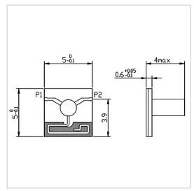
RF Solution offer a wide selection of Microstrip Isolator for global customers. MG0505-06 is a Microstrip Isolator in Frequency Range of 28.5~30.0 GHz. It is made of high quality materials under a high standard, the Insertion Loss Max of this product is 0.60 dB, Isolation Min is 17.0 dB and VSWR Max is 1.35. The component has a good working performance and stability, it is ideal for handling a Forward Power of 1 W.
