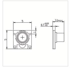
RF Solution offer a wide selection of Microstrip Isolator for global customers. MG0505-07 is a Microstrip Isolator in Frequency Range of 10.7~12.7 GHz. It is made of high quality materials under a high standard, the Insertion Loss Max of this product is 0.50 dB, Isolation Min is 20.0 dB and VSWR Max is 1.25. The component has a good working performance and stability, it is ideal for handling a Forward Power of 10 W.
