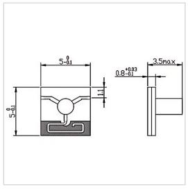
RF Solution offer a wide selection of Microstrip Isolator for global customers. MG0505-08-X-25.0-31.0GHz is a Microstrip Isolator in Frequency Range of 25.0~31.0 GHz. It is made of high quality materials under a high standard, the Insertion Loss Max of this product is 1.20 dB, Isolation Min is 15.0 dB and VSWR Max is 1.50. The component has a good working performance and stability, it is ideal for handling a Forward Power of 2 W.
