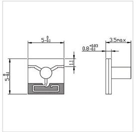
RF Solution offer a wide selection of Microstrip Isolator for global customers. MG0505-08 is a Microstrip Isolator in Frequency Range of 17.7~23.55 GHz. It is made of high quality materials under a high standard, the Insertion Loss Max of this product is 0.90 dB, Isolation Min is 15.0 dB and VSWR Max is 1.50. The component has a good working performance and stability, it is ideal for handling a Forward Power of 2 W.
