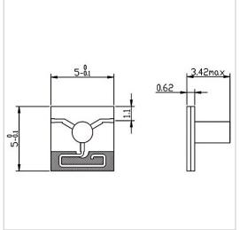
RF Solution offer a wide selection of Microstrip Isolator for global customers. MG0505-62 is a Microstrip Isolator in Frequency Range of 27.0~31.0 GHz. It is made of high quality materials under a high standard, the Insertion Loss Max of this product is 1.00 dB, Isolation Min is 18.0 dB and VSWR Max is 1.40. The component has a good working performance and stability, it is ideal for handling a Forward Power of 1 W.
