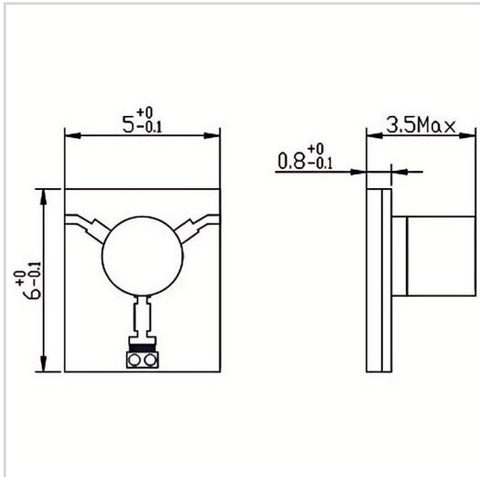
RF Solution offer a wide selection of Microstrip Isolator for global customers. MG0506-08 is a Microstrip Isolator in Frequency Range of 17.0~22.0 GHz. It is made of high quality materials under a high standard, the Insertion Loss Max of this product is 0.60 dB, Isolation Min is 16.0 dB and VSWR Max is 1.30. The component has a good working performance and stability, it is ideal for handling a Forward Power of 5 W.
