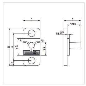
RF Solution offer a wide selection of Microstrip Isolator for global customers. MG0511-10 is a Microstrip Isolator in Frequency Range of 27.0~31.0 GHz. It is made of high quality materials under a high standard, the Insertion Loss Max of this product is 0.70 dB, Isolation Min is 17.0 dB and VSWR Max is 1.40. The component has a good working performance and stability, it is ideal for handling a Forward Power of 1 W.
