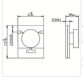
RF Solution offer a wide selection of Microstrip Isolator for global customers. MG0675-09 is a Microstrip Isolator in Frequency Range of 10.7~12.7 GHz. It is made of high quality materials under a high standard, the Insertion Loss Max of this product is 0.50 dB, Isolation Min is 18.0 dB and VSWR Max is 1.30. The component has a good working performance and stability, it is ideal for handling a Forward Power of 10 W.
