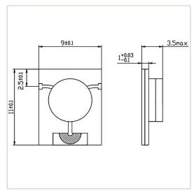
RF Solution offer a wide selection of Microstrip Isolator for global customers. MG0911-10 is a Microstrip Isolator in Frequency Range of  $5.0\sim7.0$  GHz. It is made of high quality materials under a high standard, the Insertion Loss Max of this product is 0.40 dB, Isolation Min is 20.0 dB and VSWR Max is 1.20. The component has a good working performance and stability, it is ideal for handling a Forward Power of 50 W.
