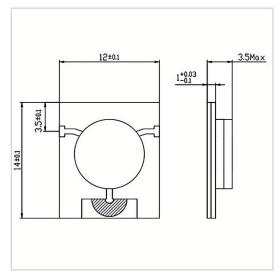
RF Solution offer a wide selection of Microstrip Isolator for global customers. MG1214-10 is a Microstrip Isolator in Frequency Range of 2.7~8.0 GHz. It is made of high quality materials under a high standard, the Insertion Loss Max of this product is 0.40~0.80 dB, Isolation Min is 14.0~20.0 dB and VSWR Max is 1.00~1.50. The component has a good working performance and stability, it is ideal for handling a Forward Power of 50 W.
