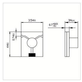
RF Solution offer a wide selection of Microstrip Isolator for global customers. MG3504-07 is a Microstrip Isolator in Frequency Range of 18.5~25.0 GHz. It is made of high quality materials under a high standard, the Insertion Loss Max of this product is 0.50~0.60 dB, Isolation Min is 24.0~41.5 dB and VSWR Max is 1.30~1.45. The component has a good working performance and stability, it is ideal for handling a Forward Power of 10 W.
