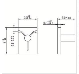
RF Solution offer a wide selection of Microstrip Isolator for global customers. MG3505-06 is a Microstrip Isolator in Frequency Range of 26.0~40.0 GHz. It is made of high quality materials under a high standard, the Insertion Loss Max of this product is 1.20 dB, Isolation Min is 11.0 dB and VSWR Max is 1.60. The component has a good working performance and stability, it is ideal for handling a Forward Power of 4 W.
