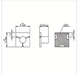
RF Solution offer a wide selection of Microstrip Circulator for global customers. MH0404-00 is a Microstrip Circulator in Frequency Range of 25.0~27.0 GHz. It is made of high quality materials under a high standard, the Bandwidth Max of this product is 100%, Insertion Loss Max is 1.10 dB and Isolation Min is 18.0 dB. The component has a good working performance and stability, it is ideal for handling a Forward Power of 20W.
