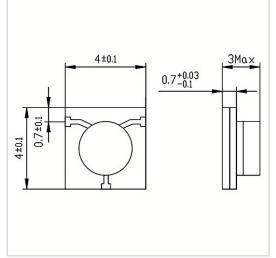
RF Solution offer a wide selection of Microstrip Circulator for global customers. MH0404-07 is a Microstrip Circulator in Frequency Range of 25.0~27.0 GHz. It is made of high quality materials under a high standard, the Bandwidth Max of this product is 40%, Insertion Loss Max is 1.10 dB and Isolation Min is 18.0 dB. The component has a good working performance and stability, it is ideal for handling a Peak Power W@ Duty Cycle 25% of 2 W.
