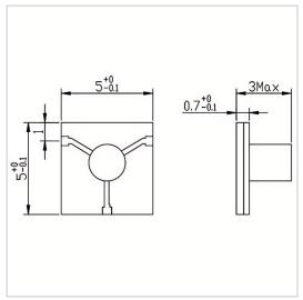
RF Solution offer a wide selection of Microstrip Circulator for global customers. MH0505-07-15-17 is a Microstrip Circulator in Frequency Range of 15.0~17.0 GHz. It is made of high quality materials under a high standard, the Bandwidth Max of this product is 100%, Insertion Loss Max is 0.40 dB and Isolation Min is 20.0 dB. The component has a good working performance and stability, it is ideal for handling a Forward Power of 10 W.
