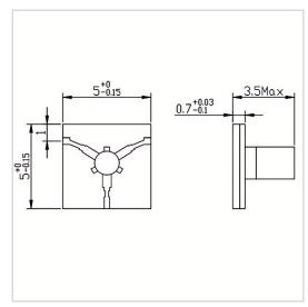
RF Solution offer a wide selection of Microstrip global Circulator for customers. MH0505-07-24.5-26.5 is a Microstrip Circulator in Frequency Range of 24.5~26.5 GHz. It is made of high quality materials under a high standard, the Bandwidth Max of this product is 100%, Insertion Loss Max is 0.50 dB and Isolation Min is 18.0 dB. The component has a good working performance and stability, it is ideal for handling a Forward Power of 10 W.
