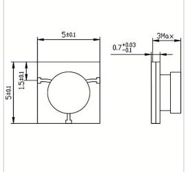
RF Solution offer a wide selection of Microstrip Circulator for global customers. MH0505-07 is a Microstrip Circulator in Frequency Range of 11.0~18.0 GHz. It is made of high quality materials under a high standard, the Bandwidth Max of this product is 20%, Insertion Loss Max is 0.50 dB and Isolation Min is 20.0 dB. The component has a good working performance and stability, it is ideal for handling a Peak Power W@ Duty Cycle 25% of 20 W.
