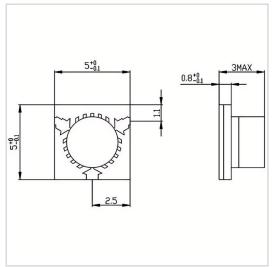
RF Solution offer a wide selection of Microstrip Circulator for global customers. MH0505-08-10-15 is a Microstrip Circulator in Frequency Range of 10.0~15.0 GHz. It is made of high quality materials under a high standard, the Bandwidth Max of this product is 100%, Insertion Loss Max is 0.60 dB and Isolation Min is 16.0 dB. The component has a good working performance and stability, it is ideal for handling a Forward Power of 2.5 W.
