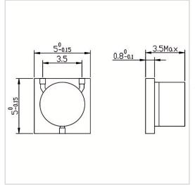
RF Solution offer a wide selection of Microstrip Circulator for global customers. MH0505-08 is a Microstrip Circulator in Frequency Range of 8.0~11.0 GHz. It is made of high quality materials under a high standard, the Bandwidth Max of this product is 100%, Insertion Loss Max is 0.50 dB and Isolation Min is 17.5 dB. The component has a good working performance and stability, it is ideal for handling a Forward Power of 10 W.
