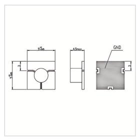
RF Solution offer a wide selection of Microstrip Circulator for global customers. MH0606-04 is a Microstrip Circulator in Frequency Range of 17.3~17.48 GHz. It is made of high quality materials under a high standard, the Bandwidth Max of this product is 100%, Insertion Loss Max is 0.70 dB and Isolation Min is 20.0 dB. The component has a good working performance and stability, it is ideal for handling a Forward Power of 10 W.
