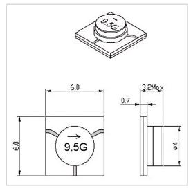
RF Solution offer a wide selection of Microstrip Circulator for global customers. MH0606-07-8-11 is a Microstrip Circulator in Frequency Range of  $8.0 \sim 11.0$  GHz. It is made of high quality materials under a high standard, the Bandwidth Max of this product is 100%, Insertion Loss Max is  $0.40 \sim 0.80$  dB and Isolation Min is  $15.0 \sim 20.0$  dB. The component has a good working performance and stability, it is ideal for handling a Forward Power of 50 W.
