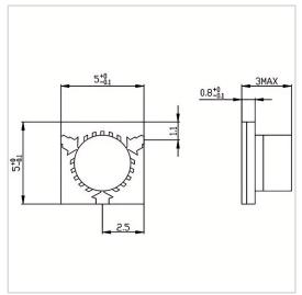
RF Solution offer a wide selection of Microstrip Circulator for global customers. MH0606-07-8-12 is a Microstrip Circulator in Frequency Range of 8.0~12.0 GHz. It is made of high quality materials under a high standard, the Bandwidth Max of this product is 100%, Insertion Loss Max is 0.60 dB and Isolation Min is 16.0 dB. The component has a good working performance and stability, it is ideal for handling a Peak Power W@ Duty Cycle 25% of 40 W.
