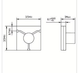
RF Solution offer a wide selection of Microstrip Circulator for global customers. MH3535-07 is a Microstrip Circulator in Frequency Range of 24.0~41.5 GHz. It is made of high quality materials under a high standard, the Bandwidth Max of this product is 100%, Insertion Loss Max is 0.60~1.00 dB and Isolation Min is 15.0~20.0 dB. The component has a good working performance and stability, it is ideal for handling a Forward Power of 10 W.
