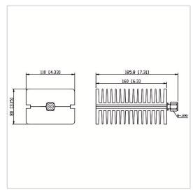
RF Solution offer a wide selection of Coaxial Mismatch Termination for global customers. MT-100WXX-F1116-NJ-XXG is a Coaxial Mismatch Termination in Frequency Range of F0±5% (F0 is the center frequency). It is made of high quality materials under a high standard, the VSWR Max of this product is 1.50~4.00, VSWR Tolerance is ±5% and Impedance is 50  $\Omega$ . The component has a good working performance and stability, it is ideal for handling a Power of 100 W.
