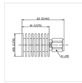
RF Solution offer a wide selection of Coaxial Mismatch Termination for global customers. MT-10WXX-R3540-NJ-XXG is a Coaxial Mismatch Termination in Frequency Range of F0±5% (F0 is the center frequency). It is made of high quality materials under a high standard, the VSWR Max of this product is  $1.50 \sim 4.00$ , VSWR Tolerance is  $\pm 5\%$  and Impedance is  $50 \Omega$ . The component has a good working performance and stability, it is ideal for handling a Power of 10 W.
