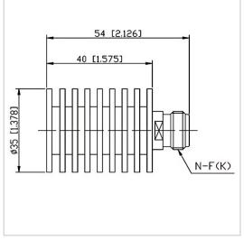
RF Solution offer a wide selection of Coaxial Mismatch Termination for global customers. MT-10WXX-R3540-NK-XXG is a Coaxial Mismatch Termination in Frequency Range of F0±5% (F0 is the center frequency). It is made of high quality materials under a high standard, the VSWR Max of this product is 1.50~4.00, VSWR Tolerance is ±5% and Impedance is 50  $\Omega$ . The component has a good working performance and stability, it is ideal for handling a Power of 10 W.
