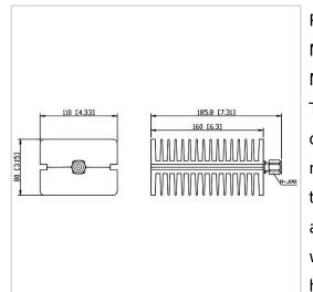
RF Solution offer a wide selection of Coaxial Mismatch Termination for global customers. MT-150WXX-F1116-NJ-XXG is a Coaxial Mismatch Termination in Frequency Range of F0±5% (F0 is the center frequency). It is made of high quality materials under a high standard, the VSWR Max of this product is  $1.50 \sim 4.00$ , VSWR Tolerance is  $\pm 5\%$  and Impedance is 50  $\Omega$ . The component has a good working performance and stability, it is ideal for handling a Power of 150 W.
