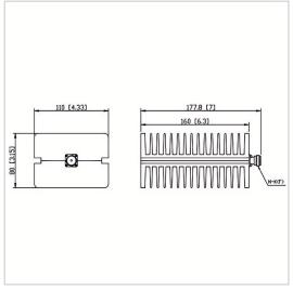
RF Solution offer a wide selection of Coaxial Mismatch Termination for global customers. MT-150WXX-F1116-NK-XXG is a Coaxial Mismatch Termination in Frequency Range of F0 $\pm$ 5% (F0 is the center frequency). It is made of high quality materials under a high standard, the VSWR Max of this product is 1.50~4.00, VSWR Tolerance is  $\pm$ 5% and Impedance is 50  $\Omega$ . The component has a good working performance and stability, it is ideal for handling a Power of 150 W.
