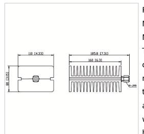
RF Solution offer a wide selection of Coaxial Mismatch Termination for global customers. MT-200WXX-F1116-NJ-XXG is a Coaxial Mismatch Termination in Frequency Range of F0±5% (F0 is the center frequency). It is made of high quality materials under a high standard, the VSWR Max of this product is  $1.50 \sim 4.00$ , VSWR Tolerance is  $\pm 5\%$  and Impedance is  $50 \Omega$ . The component has a good working performance and stability, it is ideal for handling a Power of 200 W.
