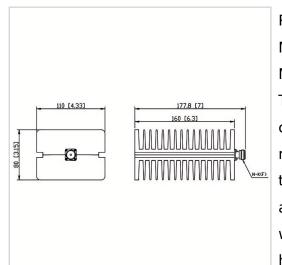
RF Solution offer a wide selection of Coaxial Mismatch Termination for global customers. MT-200WXX-F1116-NK-XXG is a Coaxial Mismatch Termination in Frequency Range of F0±5% (F0 is the center frequency). It is made of high quality materials under a high standard, the VSWR Max of this product is  $1.50 \sim 4.00$ , VSWR Tolerance is  $\pm 5\%$  and Impedance is  $50 \Omega$ . The component has a good working performance and stability, it is ideal for handling a Power of 200 W.
