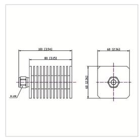
RF Solution offer a wide selection of Coaxial Mismatch Termination for global customers. MT-50WXX-F6080-NJ-XXG is a Coaxial Mismatch Termination in Frequency Range of F0±5% (F0 is the center frequency). It is made of high quality materials under a high standard, the VSWR Max of this product is 1.50~4.00, VSWR Tolerance is ±5% and Impedance is 50  $\Omega$ . The component has a good working performance and stability, it is ideal for handling a Power of 50 W.
