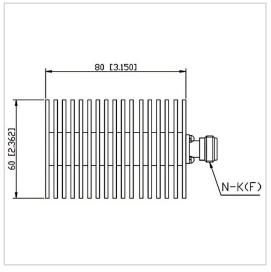
RF Solution offer a wide selection of Coaxial Mismatch Termination for global customers. MT-50WXX-F6080-NK-XXG is a Coaxial Mismatch Termination in Frequency Range of F0 $\pm$ 5% (F0 is the center frequency). It is made of high quality materials under a high standard, the VSWR Max of this product is 1.50~4.00, VSWR Tolerance is  $\pm$ 5% and Impedance is 50  $\Omega$ . The component has a good working performance and stability, it is ideal for handling a Power of 50 W.
