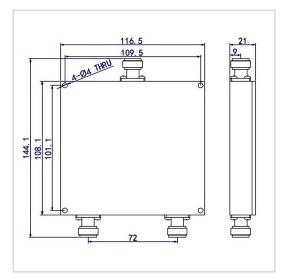
RF Solution offer a wide selection of 2 Ways Power Divider for global customers. PD02-F1211-N-80-900MHz is a 2 Ways Power Divider in Frequency Range of 80~900 MHz. It is made of high quality materials under a high standard, the Split Loss of this product is 3.0 dB, Insertion Loss Max is 0.7 dB and Isolation Min is 15.0 dB. The component has a good working performance and stability, it is ideal for handling a Rated Power of 25 W.
