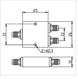
RF Solution offer a wide selection of 2 Ways Power Divider for global customers. PD02-F2625-S-18-40GHz is a 2 Ways Power Divider in Frequency Range of  $18.0 \sim 40.0$  GHz. It is made of high quality materials under a high standard, the Insertion Loss Max of this product is 1.2 dB, Isolation Min is 16 dB and Amplitude Unbalance is  $\pm 0.4$  dB. The component has a good working performance and stability, it is ideal for handling a Forward Power of 20 W.
