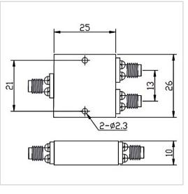
RF Solution offer a wide selection of 2 Ways Power Divider for global customers. PD02-F2625-S-27-32GHz is a 2 Ways Power Divider in Frequency Range of  $18.0 \sim 40.0$  GHz. It is made of high quality materials under a high standard, the Insertion Loss Max of this product is 1.0 dB, Isolation Min is 18 dB and Amplitude Unbalance is  $\pm 0.4$  dB. The component has a good working performance and stability, it is ideal for handling a Forward Power of 20 W.
