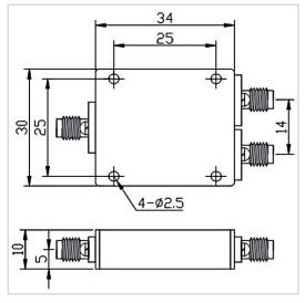
RF Solution offer a wide selection of 2 Ways Power Divider for global customers. PD02-F3034-S-2-6GHz is a 2 Ways Power Divider in Frequency Range of  $2.0\sim6.0$  GHz. It is made of high quality materials under a high standard, the Insertion Loss Max of this product is 0.5 dB, Isolation Min is 20 dB and Amplitude Unbalance is  $\pm0.3$  dB. The component has a good working performance and stability, it is ideal for handling a Forward Power of 30 W.
