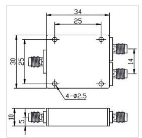
RF Solution offer a wide selection of 2 Ways Power Divider for global customers. PD02-F3034-S-2-8GHz is a 2 Ways Power Divider in Frequency Range of 2.0~8.0 GHz. It is made of high quality materials under a high standard, the Insertion Loss Max of this product is 0.6 dB, Isolation Min is 20 dB and Amplitude Unbalance is  $\pm 0.3$  dB. The component has a good working performance and stability, it is ideal for handling a Forward Power of 20 W.
